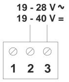
The power supply voltage must be in the range of 19 to 40 VDC (any polarity or 19 and 28 VAC; also see *INSTALLATION* section.
