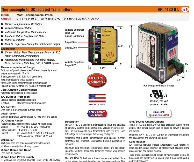
20 VDC nominal, regulated, 25 mADC, max. ripple <10 mVRMs EXTSUP option: Unpowered mA output
