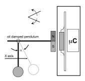
Pendulum damping: by oil filling
