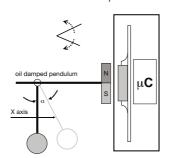
Pendulum damping: by oil filling
