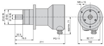
Fig. 8. KINAX WT 717 with flange.
