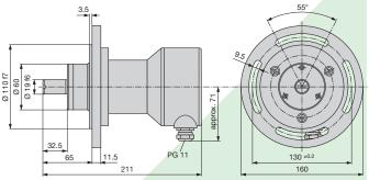
Fig. 10. KINAX WT 717 with additional gear and foot.
