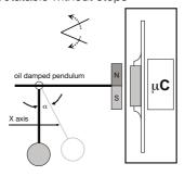
Pendulum damping: by oil filling
