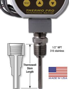
See thermowell manufacturer's specifications. Probe length is measured from top of full threads to tip of probe.
