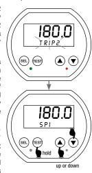
Note that the unit will not respond to changes in temperature, LEDs are turned off, and the alarm relays will maintain their prior states while the TEST button is held.
