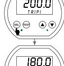
When the Trip Point 1 value is being displayed, press and release the SEL button. The Trip Point 2 value will be displayed with TRIP2 on the lower display.
