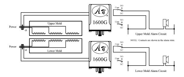
NOTE: During the normal ON/OFF cycle of the temperature controller the low current alarm will cycle with the heater. When the alarm fails to reset as the heaters are turned back on or if an alarm indication occurs during the "heat" cycle one or more of the heaters have failed.
